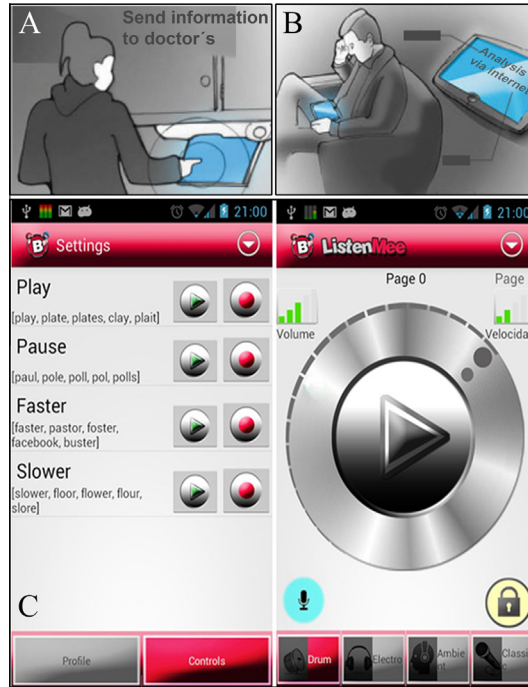
Fig. 2. Listenmee ® App (C and D) the interface used is simple employing a circle type up button touch screen ordering system with commands such as “PLAY”, “PAUSE”. The user is able to increase (clockwise) or decrease (against clockwise) the cueing rate. It has 4 special categories identified as: “environmental”, “drums”, “electronics”, “voices”. Furthermore each category has 25 different sounds, for a total of 100 sounds. Listenmee ® and Listenmee app ® have a statistical analyses software, recording walking improvement in daily traveled distances and time scores (A and B). The user walking route performances can be recorded daily, monthly and annually by integrating the prototype and app and existing monitor maps (GPS). The physician can access the patient scores data through Internet at all times through telemedicine.
